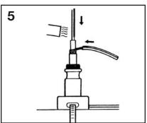
Slide the black 1/8" x 51/2" heatshrink tubes on the bus wires, and the green/vellow 1/4" x 51/2" heat-shrink tube on the ground pigtail. Heat shrink, using a heat gun, or soft flame torch, moving the heat source back and forth.
