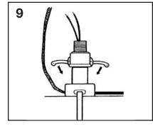
Slide the top in place and push and lock the cam levers into position. Lock cam levers in place by inserting the stainless steel tie wire through the holes in the ends of the cam levers and twisting together.
