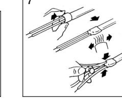
Slide the white  $1/2" \times 11/2"$  heatshrink tube in place over the bus wires and onto the inner jacket. Heat shrink in place. After removing the heat source, and while still hot, pinch the center of the heat-shrink tube between the bus wires with needle-nose pliers.
