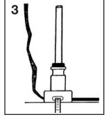
Extend the heater 71/2" above the base. Allow braid pigtail to extend out from bottom of base. Attach base to pipe with a pipe strap. Slide the grommet over the heater and push into cavity in base
