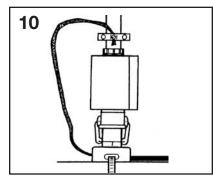
Mount junction box with non-threaded opening for 3/4" conduit, using the sealing gasket and lock ring to hold in place, or use a junction box with a 3/4" inside threaded hub. Ground the braid pigtail to conduit with a clamp (not provided).
