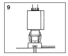
Mount junction box with non-threaded opening for 3/4" conduit, using the sealing gasket and lock ring to hold in place, or use a junction box with a 3/4" inside threaded hub.
