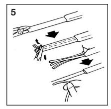
Notch the center core between the conductors and pull the bus wires away from the core for 6". Remove the center core material and any core material on the bus wires. Retwist the bus wires, if needed.
