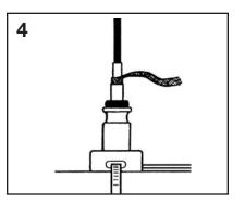
Strip the inner jacket 6" from the end. Strip the bus wires out of the core, following the Heat Trace Stripping Instructions.
