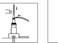
Slide the white 1/2" x 11/2" heatshrink tube in place over the bus wires and onto the inner jacket. Heat shrink in place. After removing the heat source, and while still hot. pinch the center of the heat-shrink tube between the bus wires with needle-nose pliers.
