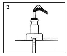
Make an opening in the ground braid, bend the heater, and pull the inner jacket and core through the opening in the braid. Twist the around braid into a pigtail.
