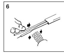
Slide the black 1/8" x 51/2" heatshrink tubes on the bus wires, and the green/yellow 1/4" x 51/2" heat-shrink tube on the ground pigtail. Heat shrink, using a heat gun, or soft flame torch.
