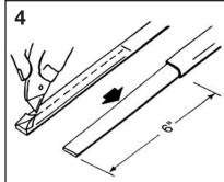
Strip the jacket 6" from the end to expose the conductive core.
