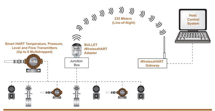
ULLE WirelessHART® Adapter for Use with Wired HART® Field Devices
