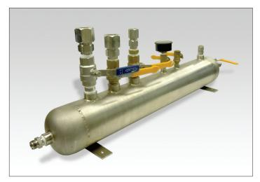
**SAGE ZEROING CHAMBER** One of the many data points taken during the Flow Meter's NIST calibration at Sage is at a "No Flow" (0 SCFM) condition. The Sage Zeroing Chamber is used to capture a "No Flow" (0 SCFM) flow point at the actual conditions (i.e., with the same gas or gas mix and same pressure as that specified by the customer for their process)
