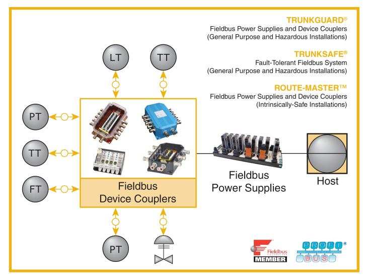
Fieldbus Device Couplers and Power Supplies deliver a fast and easy way to connect, protect, power and terminate multiple fieldbus devices in FOUNDATION fieldbus<sup>™</sup> and PROFIBUS PA segments.
