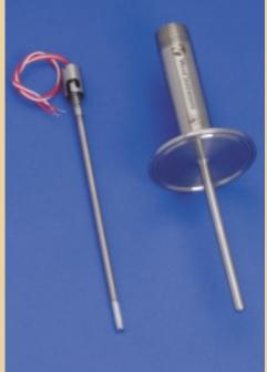
For use where sensor needs to be calibrated or replaced without shutting down the vessel system.
