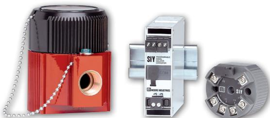
The SIY combines smart digital technology with advanced analog operation to deliver superior reliability, accuracy, and ease of use. The highly versatile SIY programs to accept a wide range of current or voltage inputs. It outputs an isolated, proportional, 4-20mA signal. As a flexible analog/digital hybrid, this 2-wire (loop-powered) transmitter programs in seconds with easy to use free software to handle a wide range of important signal interface applications.
