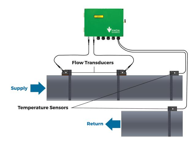
✓ All VorTek flow metering products have thermal energy metering capabilities.
