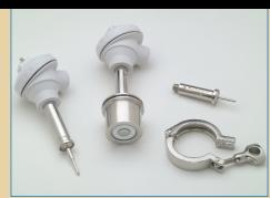
Weed Instrument sanitary RTDs, thermocouples, thermowells and temperature transmitters have been designed to meet the environmental and performance requirements of pharmaceutical and biotech processing and sterilization applications. Most sensors feature enhanced performance specifications and 316L stainless steel materials and can be electropolished to a Ra of 0.2 microns (8 microinches). Also, permanently etched tagging information and calibration certificates can be provided.
